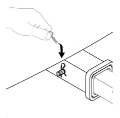
3. Remove the quick release locking pin from the mounting plate & Install the Ronin Ascender onto the mounting plate of the Ronin Trailer Hitch. Lock the Ronin Ascender into place, using the quick release locking pin.
