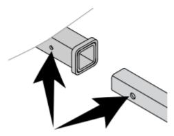
2. Line up the mounting hole and install your vehicles hitch locking pin. Be sure to secure the locking pin into place, so it does not come loose overtime with vibration or impact.
